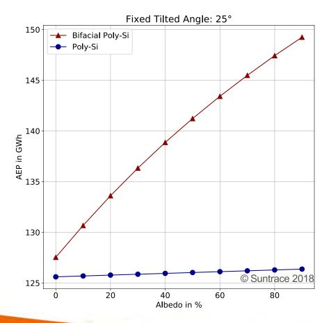
Example 50 MW AC plant in Tunesia AC/DC = 1.3
