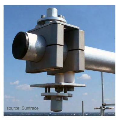
Albedometer using photodiode sensors
