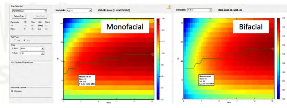
Bifacial layouts show optimum at slightly higher tilt than monofacial.
